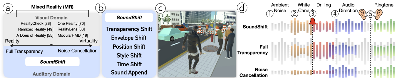
Figure 1: We present SoundShift , a concept to manipulate sounds to improve mixed-reality awareness. (a) SoundShift is situated in the auditory Reality-Virtuality Continuum with full transparency and noise cancellation as two ends, and comprises (b) six sound manipulators, which are TRANSPARENCY SHIFT, ENVELOPE SHIFT, POSITION SHIFT, STYLE SHIFT, SOUND APPEND, and TIME SHIFT. (c) In a scenario, a VBI user navigates a busy street with a white cane and audio directions. They sometimes may receive ringtones and pass by construction sites with drilling noises. (d.1) TRANSPARENCY SHIFT makes the auditory transparency half to suppress nuanced noises while retaining real-world awareness. (d.2) ENVELOPE SHIFT increases the white cane sounds to make them distinctive. (d.3) SOUND APPEND plays an earcon to signal the danger, and STYLE SHIFT applies a low-pass filter to make drilling noise less sharp to hear. (d.4) TIME SHIFT delays the audio directions when they conflict with drilling noises. (d.5) POSITION SHIFT places ringtone on the right and audio directions on the left to increase distinguishability.
