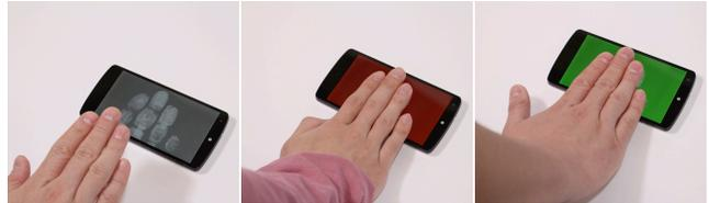
**Figure 2. CapAuth classification. Left: initial state. Middle: unauthorized user (red). Right: authorized user (green).**
