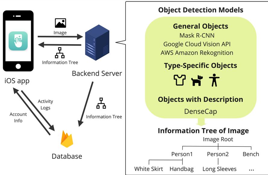
**Figure 2: ImageExplorer System Diagram.** The app sends images to the backend. The backend will process the image through a series of models and return a hierarchical information tree of the image. Firebase is used to store all relevant data.
